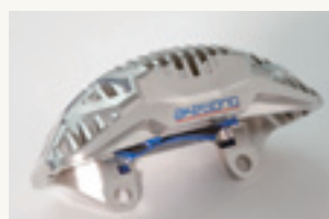
Caliper for mid-range performance vehicles: 4-pot aluminum monoblock caliper
