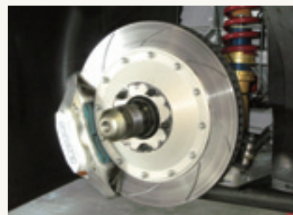
Rear caliper: four-piston monoblock caliper
