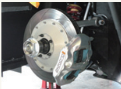
Front caliper: six-piston monoblock caliper
