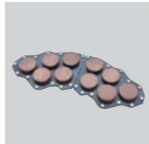
Bullet train disc brake lining
