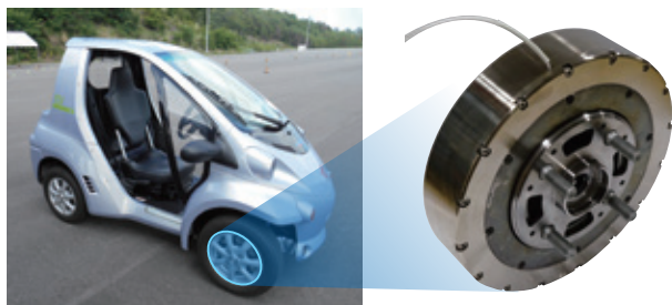
MR fluid brake prototype fitted to a small mobility vehicle
