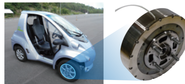
MR fluid brake (prototype) and ultra-compact mobility vehicle fitted with it
