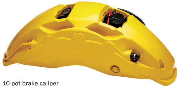
10-pot brake caliper for high-performance mass-production cars
