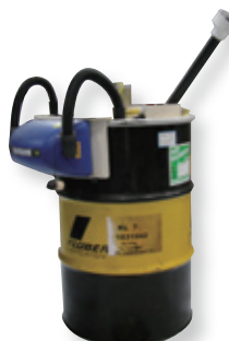
Bulb crusher: Using a triple-layer filter, this unit first separates glass, metal caps and other materials into collection receptacles, then turns mercury into an insoluble mercuric sulfide to recover it safely.
