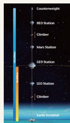
Conceptual drawing of the structure of a space elevator (Provided by JAPAN SPACE ASSOCIATION)
