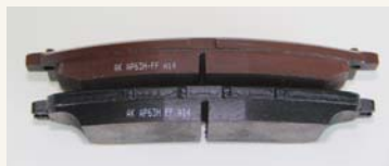
A brake pad labeled with Friction Materials Edge Code Markings
