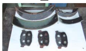
Detached drum brake shoes and disc brake pads (foreground)
