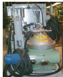
Centrifuge equipment capable of separating a type of oil that could not have been separated using the settled separation method
