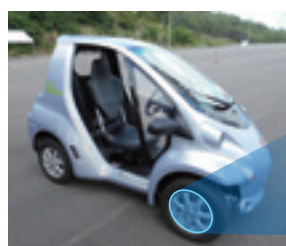
MR fluid brake (prototype) and ultra-compact mobility vehicle fitted with it
