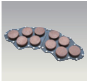
Bullet train disc brake lining
