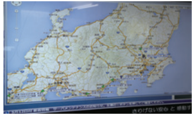
Alocs Corporation's control screen that gives driving instructions based on real-time truck position and traffic information
