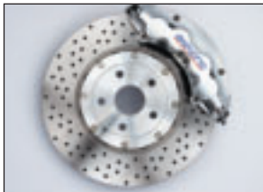
Eight-pot aluminum caliper and rotor for high-performance cars (concept)
