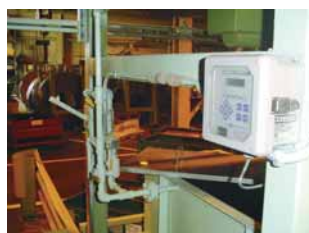
First stage rinse tank equipped with conductivity meter (ABE)
