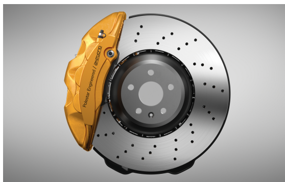
6-piston aluminum mono block opposed caliper
