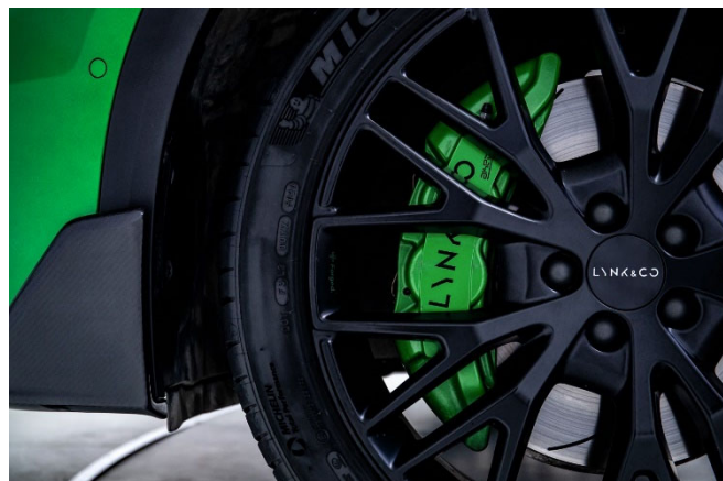
Opposed piston type 4-pot brake calipers for the Lynk & Co 05+
